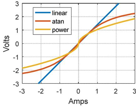
Fig. 5. Linear vs nonlinear resistor dependencies.
