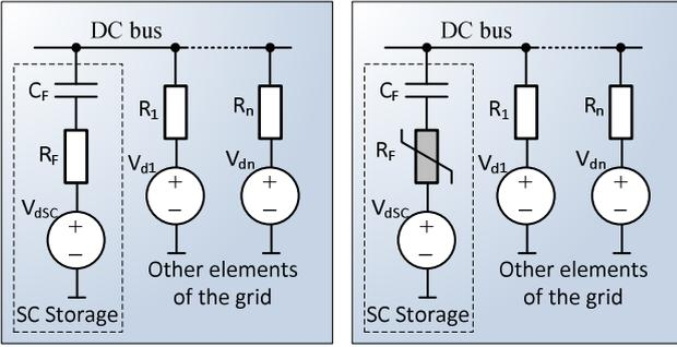
Fig. 6. Conventional EMS for SC charge (left) VS Proposed EMS (right).
