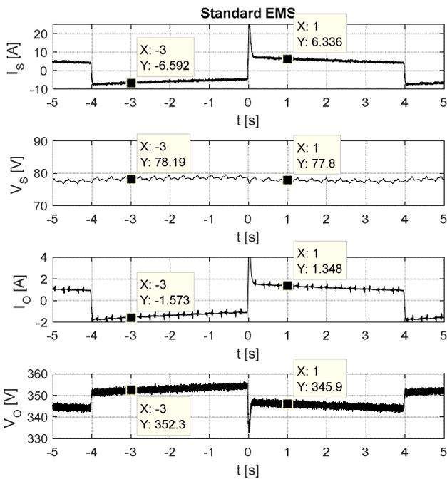
Fig. 12. Conventional EMS; Step voltage change ( $\Delta V = \pm 10$  V).
