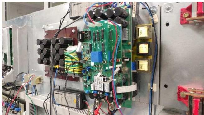
Fig. 18. High ratio converter connected to DC grid.
