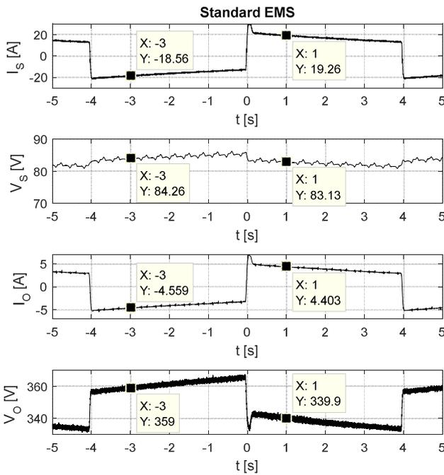
Fig. 13. Conventional EMS; Step voltage change ( $\Delta V = \pm 30$  V).
