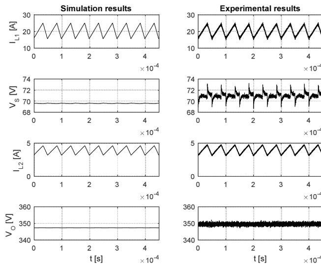
Fig. 17. Steady state waveforms for step up mode ( $I_{L1} = 20 A$ ).
