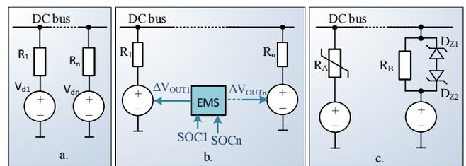
Fig. 3. Droop based control: a. Conventional; b. Centralized; c. Nonlinear.
