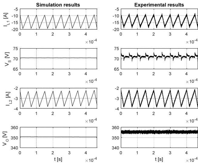
Fig. 16. Steady state waveforms for step down mode ( $I_{L1} = -15A$ ).
