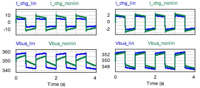
Fig. 7. Linear vs proposed EMS filtering method  $f = 1\text{Hz}$  ( $dV=30\text{V}$  - left;  $dV=10\text{V}$  - right).
