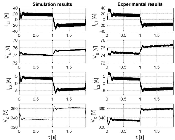
Fig. 11. SC discharge to SC charge transition (ΔV = ± 30 V).
