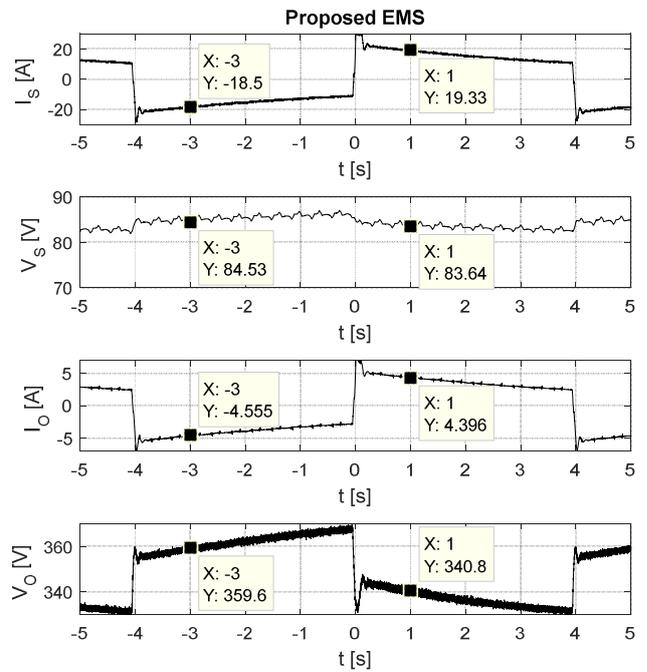
Fig. 15. Proposed EMS; Step voltage change ( $\Delta V = \pm 30$  V).
