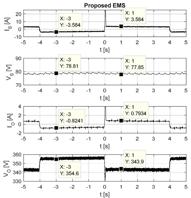
Fig. 14. Proposed EMS; Step voltage change ( $\Delta V = \pm 10$  V).
