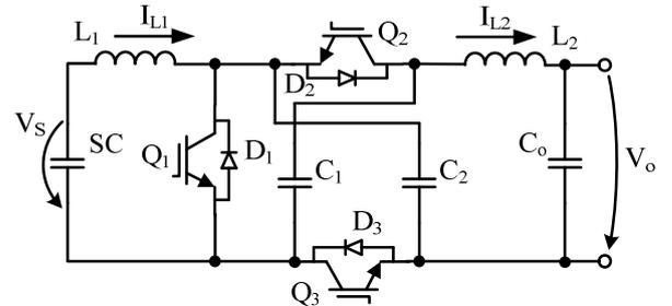
Fig. 9. DC Converter topology used for SC charging.
