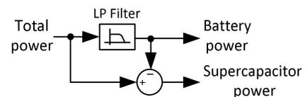
Fig. 4. Conventional filtering method used in centralized EMS.
