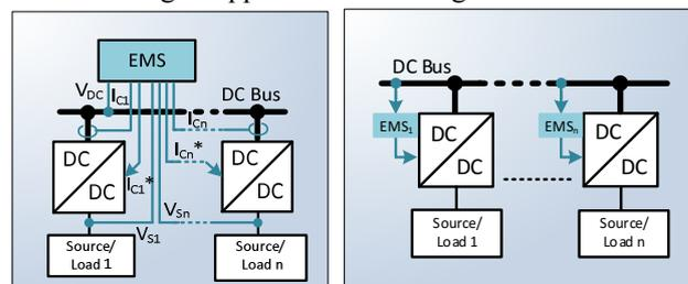
Fig. 2. Centralized EMS (left) and Decentralized EMS (right).
