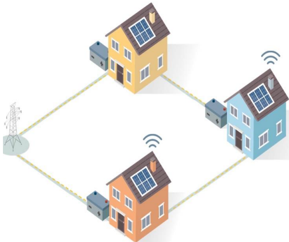
Fig. 4. SMART microgrid connected to utility grid
