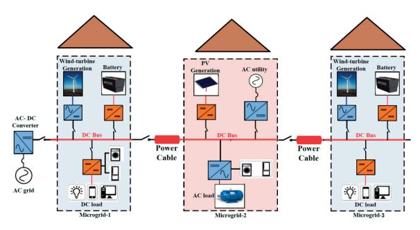
**Figure 12.**Radial DC grid topology [22].
