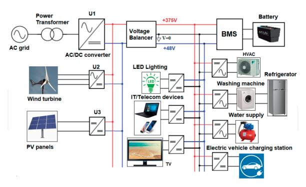
**Figure 14.**Topology of a household DC power distribution system which integrates typical consumers as well as renewable energy sources.
