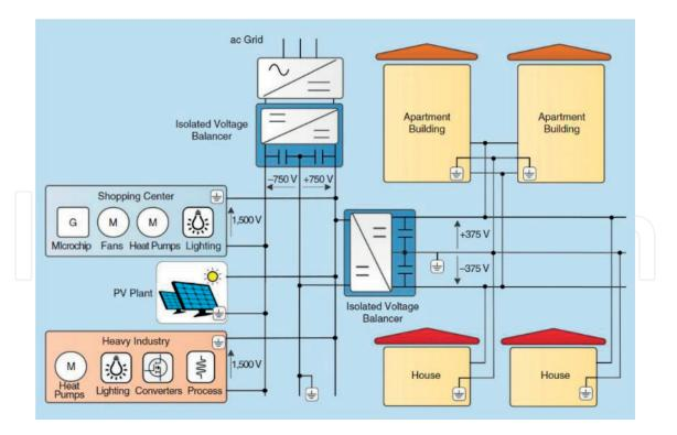
**Figure 11.**DC grid provided with multiple voltage levels [22].
