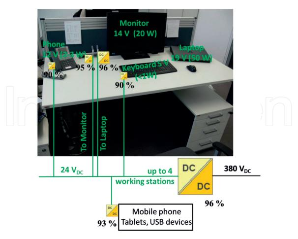
**Figure 5.**Power supply infrastructure for office equipment [18].
