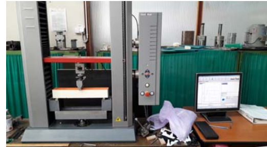
b) Three point bending test of the sample
