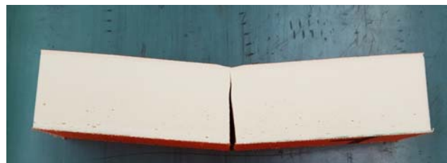
b) Failure of the tension face
