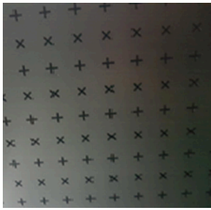
Fig. 3. Absorber (metal plate) with lobed holes.
