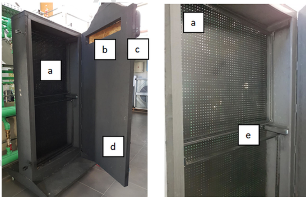
Fig. 4. TSC with PCMs (construction details), a – absorber plate; b – air opening in the top part of the TSC cavity; c – air plenum; d – TSC rear wall; e – metal frame for PCMs.
