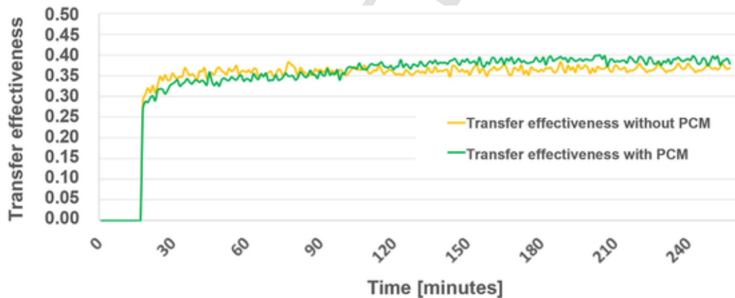
Fig. 16. Heat exchange effectiveness for TSC with/without PCM.
