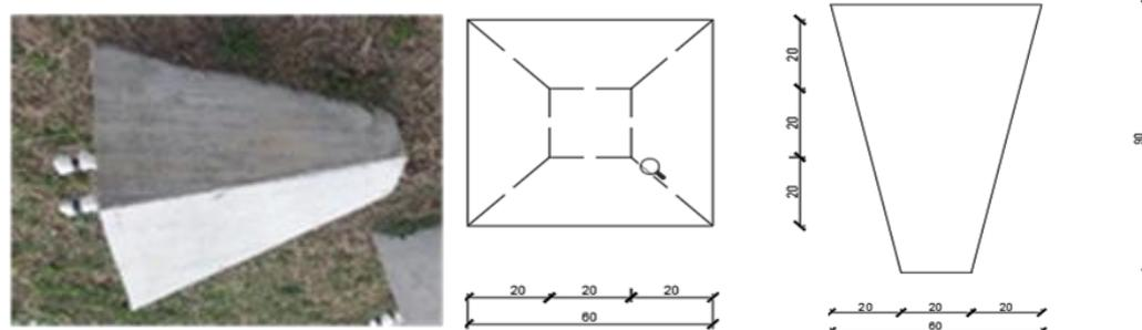
**Figure 10.** Precast wedge foundation – adapted from [29]: actual singular foundation before installation – left, singular foundation dimensions – middle and right.
