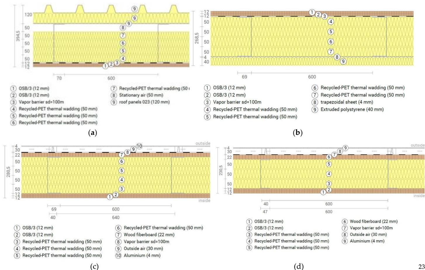
**Figure 11.** LSF construction elements stratification: (a) Roof; (b) Floor; (c) Northern wall; (d) Eastern and Western wall.
