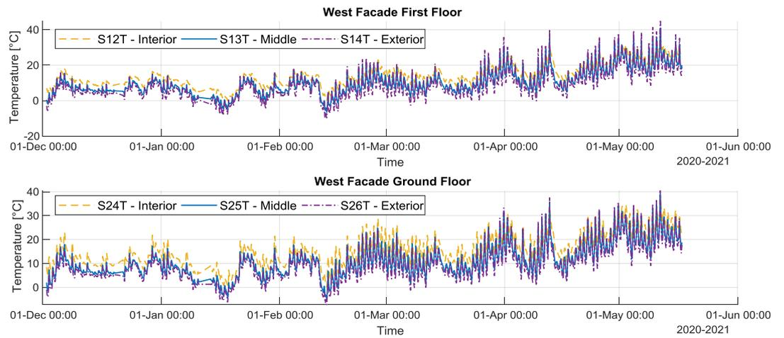
Figure 19. Temperature data provided by the sensors for the Western Façade First Floor (above) and Ground Floor (below).
