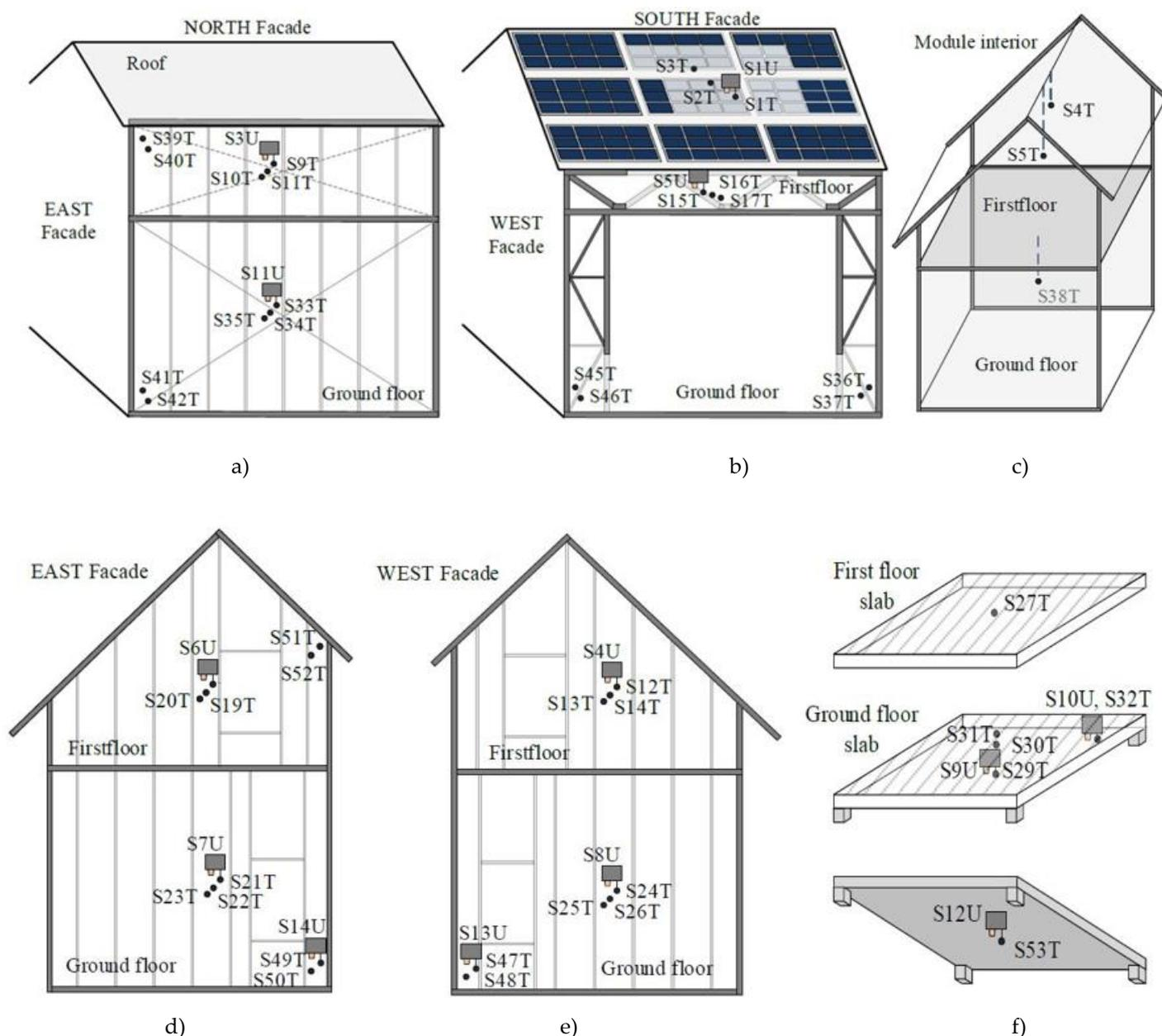
**Figure 14.** Sensors' distribution on LSF experimental module: a) North Façade b) Southern Façade and Roof c) Interior d) East Façade e) West Façade f) in slabs (adapted from [9]).
