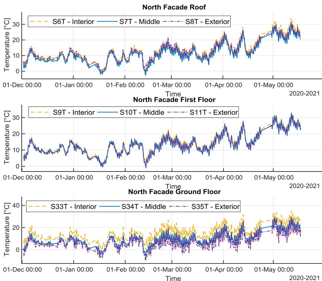
Figure 18. Temperature data provided by the sensors for the Northern side of the building: Roof 367
