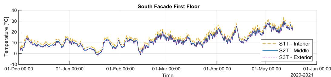
**Figure 16.** a) Temperature data provided by the sensors for Southern Façade First Floor.
