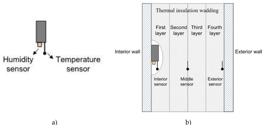
**Figure 15.** a) Humidity and temperature sensor configuration b) Sensors' distribution between thermal insulation layers.
