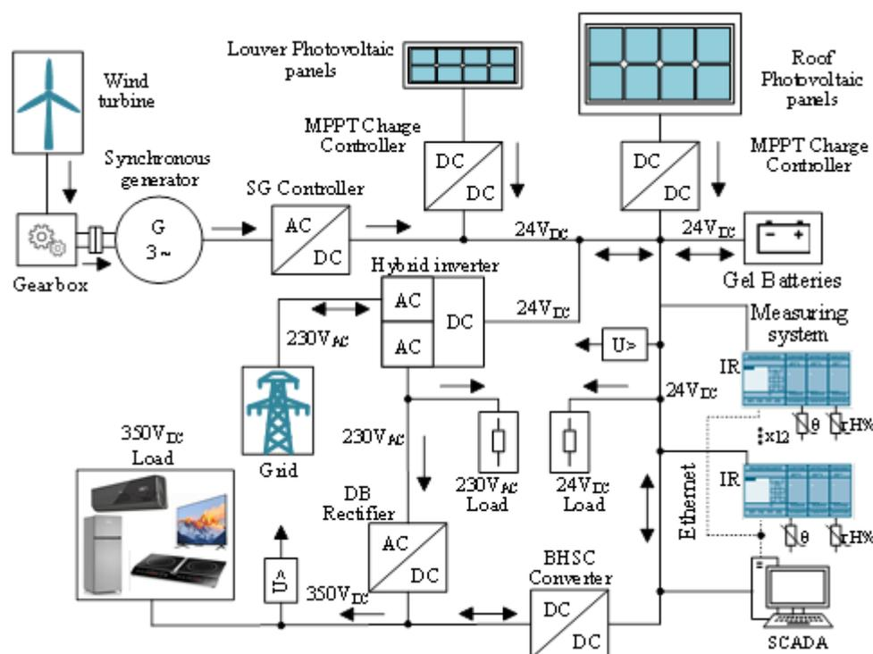
Figure 13. The architecture of the implemented smart nano-grid (adapted from [9]).
