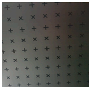
Fig. 3. Absorber (metal plate) with lobed holes.
