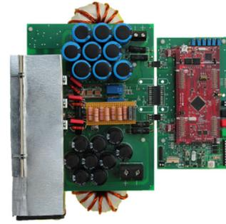
**FIGURE 31** BHSI prototype with MOSFET transistors (IXFK80N60P3)
