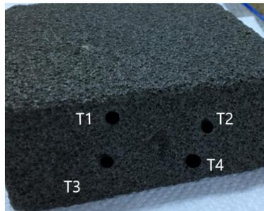
Figure 7. Image of foam glass with 4 points where temperature was measured
