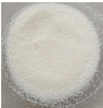
**Figure 1.** The appearance of the adsorbent material obtained by functionalizing  $\text{MgSiO}_3$  using DL-cysteine.
